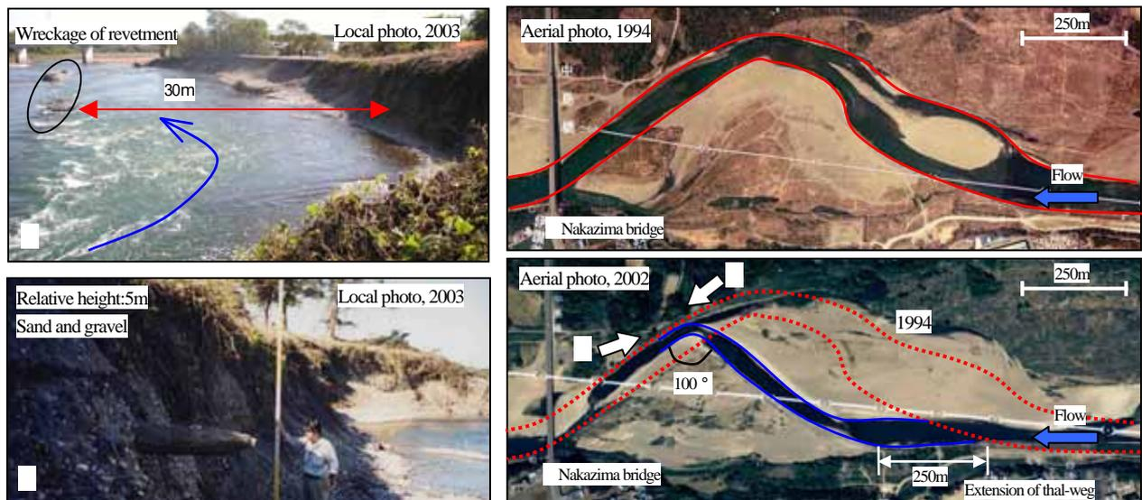
Photo 2. Development of crank flow between 1994 and 2002, and river bank erosion after suffering (2003) in Kinu-river
